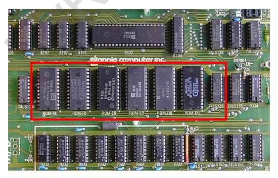
Install the ROM replacement board into sockets D0 and F12. Make sure the pins are all aligned before pressing into place.
