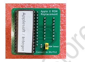
The Apple II ROM Replacement board replaces the ROMs on your Apple computer with a single ROM. The replacement ROM allows you to select either Applesoft BASIC, or Integer BASIC by using a jumper.
